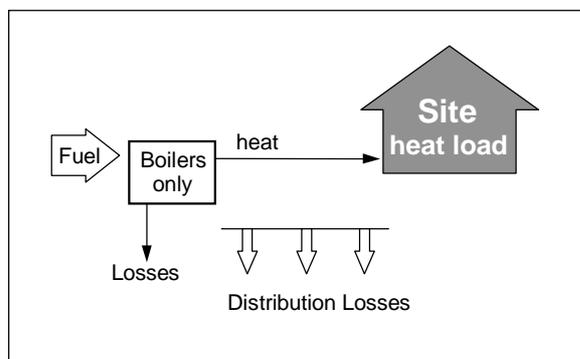
Figure C1 : Community heating with heat supplied by boilers only
