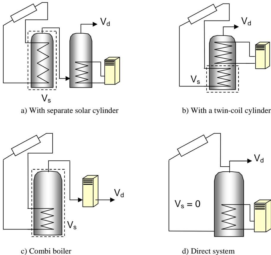
$V_s$  (indicated by the dashed line) is the dedicated solar storage volume. See text below concerning the effective solar volume.  $V_d$  is the daily hot water demand. These schematics do not include all possible arrangements and are not intended to show safety measures and devices needed to make the systems safe.
