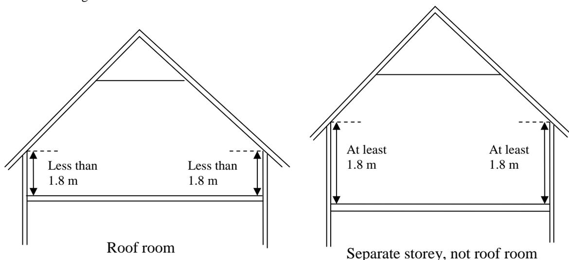
Figure S2 : Upper storey with common wall
