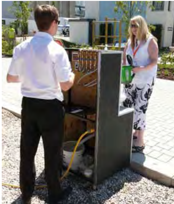
Figure 2: Specially designed test rig used to assess public opinion about low flow water fittings at BRE's Insight09 event
