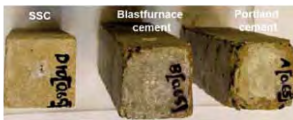
Figure 2: Observation of concretes made using SSC, blastfurnace cement and Portland cement after exposure to 5% Na 2 SO 4 for 100 weeks (w/c ratio = 0.65)
