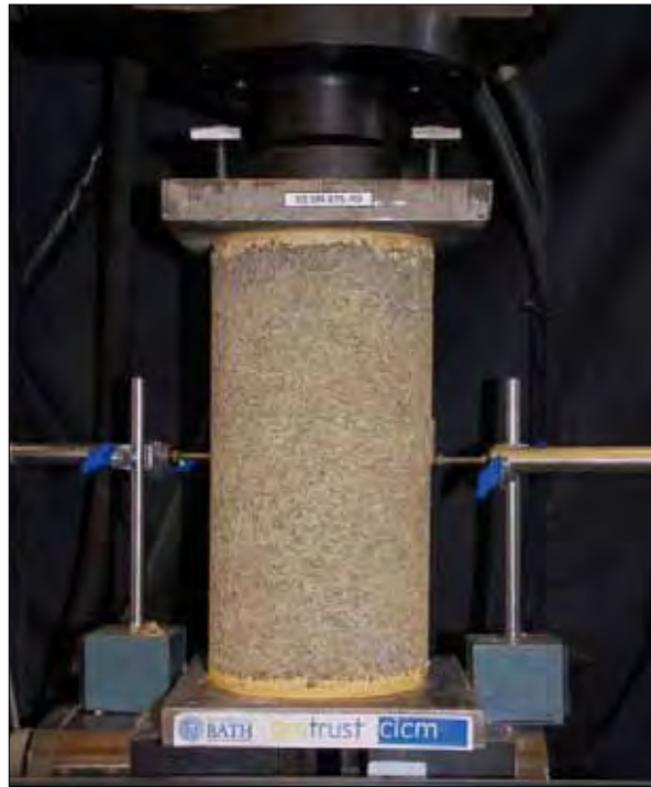
Figure 2: Compression testing of hemp-lime specimen
