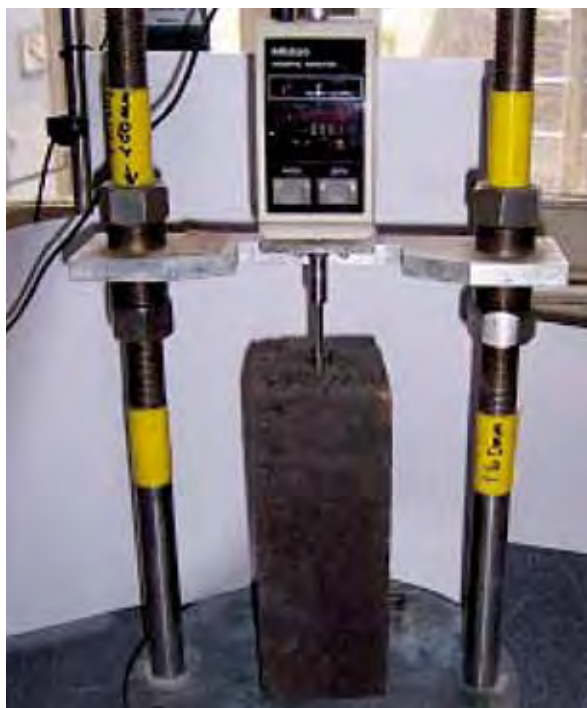
Figure 3: Measurement of expansion due to ASR
