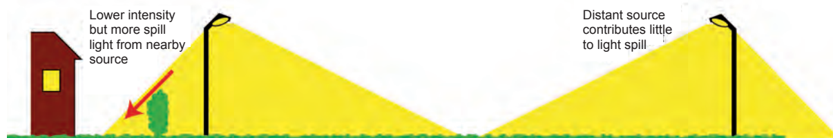
Figure 2: A problem with current guidelines based on the intensity of floodlights is that no allowance is made for the distance of the source
