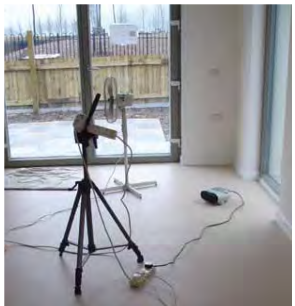
Figure 5: Co-heating setup in a low-energy dwelling. Courtesy of Shiyu Jiang
