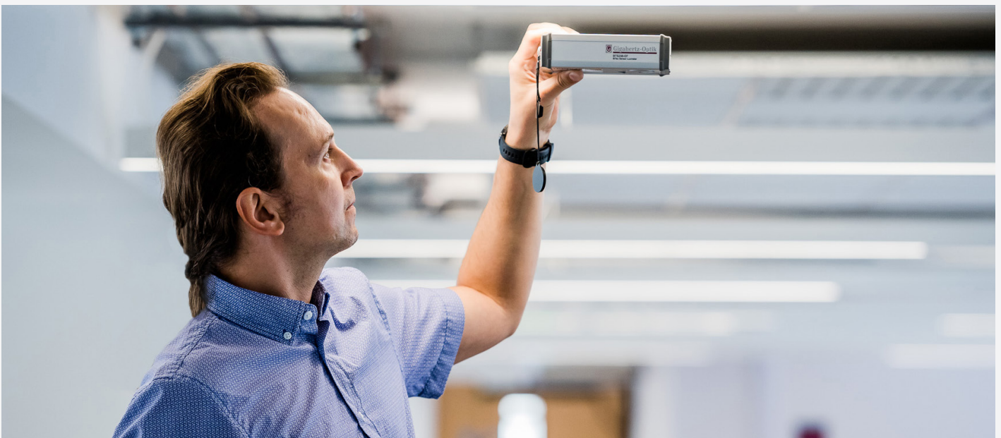
BRE expert measuring electric lighting in a building
