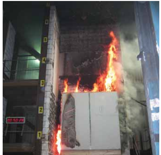
Figure 3: Fire spread to upper panel above cavity barrier
