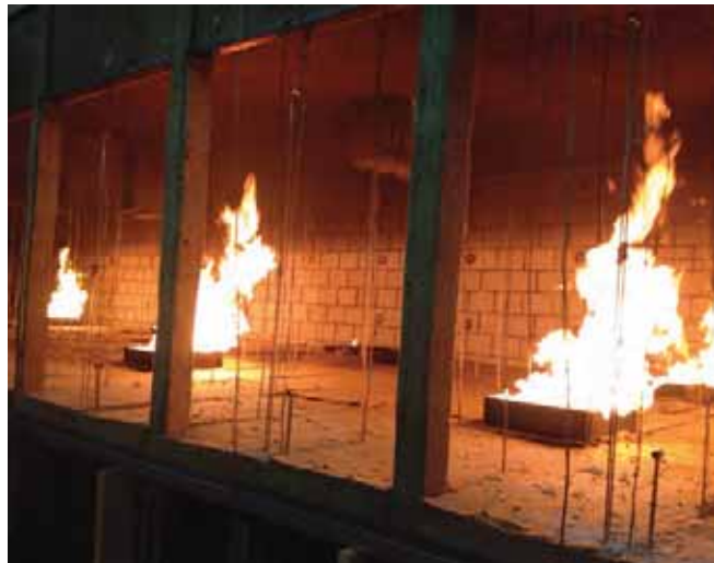
Figure 1: Burner testing is carried out in the purpose-built, heavily sensed test compartment, constructed within the Burn Hall facility at BRE's Watford site
