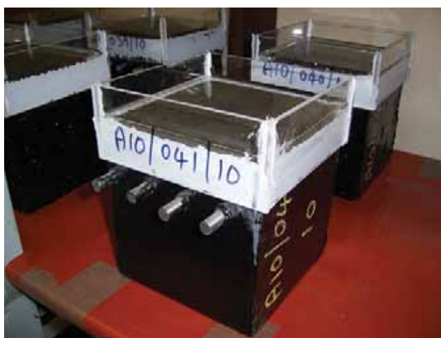
Figure 3: Reinforced concrete test specimens for ponding with chloride solution and monitoring for reinforcement corrosion
