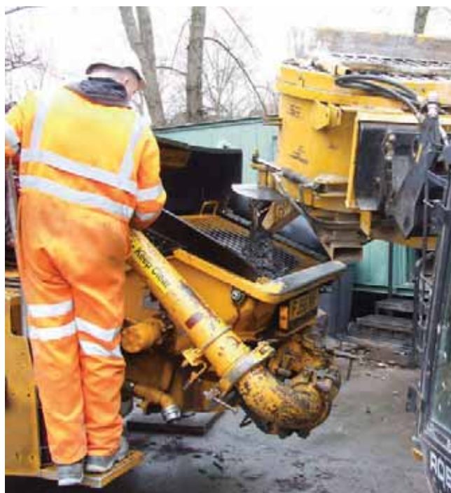
Figure 1: An industrial trial being conducted with an alkali-activated binder concrete pump concrete mix
