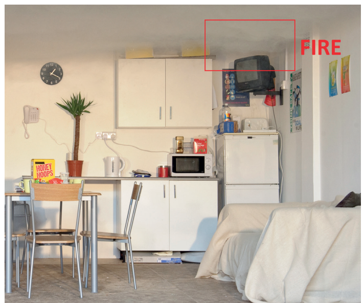
Figure 20: Fire threat detected by a video fire detection system
