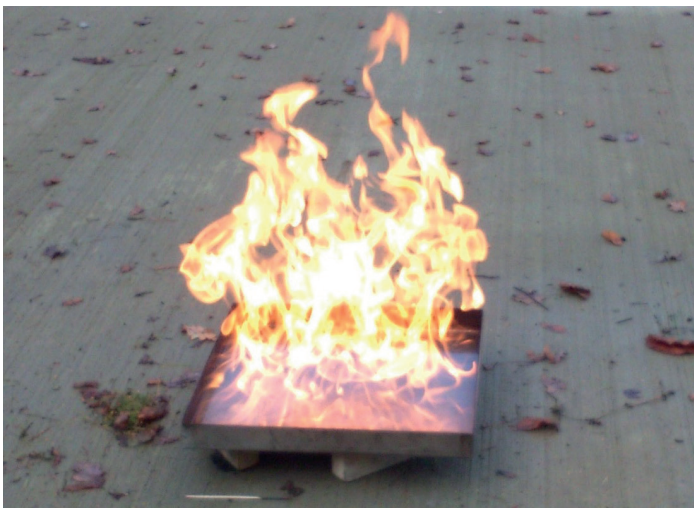
Figure 5: n-Heptane test fire in the 500mm square steel tray
