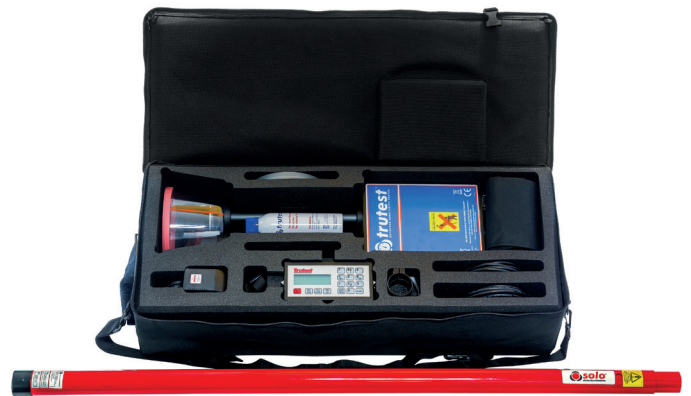
Figure 2: Trutest smoke sensitivity measurement equipment (photo courtesy of Detector Testers)
