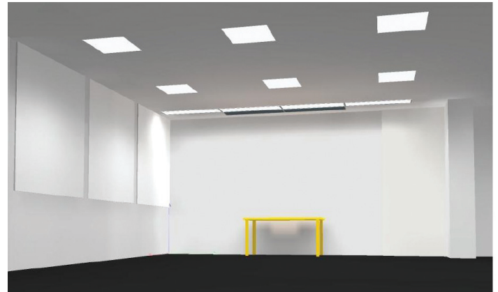
Figure 1: DIALux simulation of a space with four wall-washer light fittings
