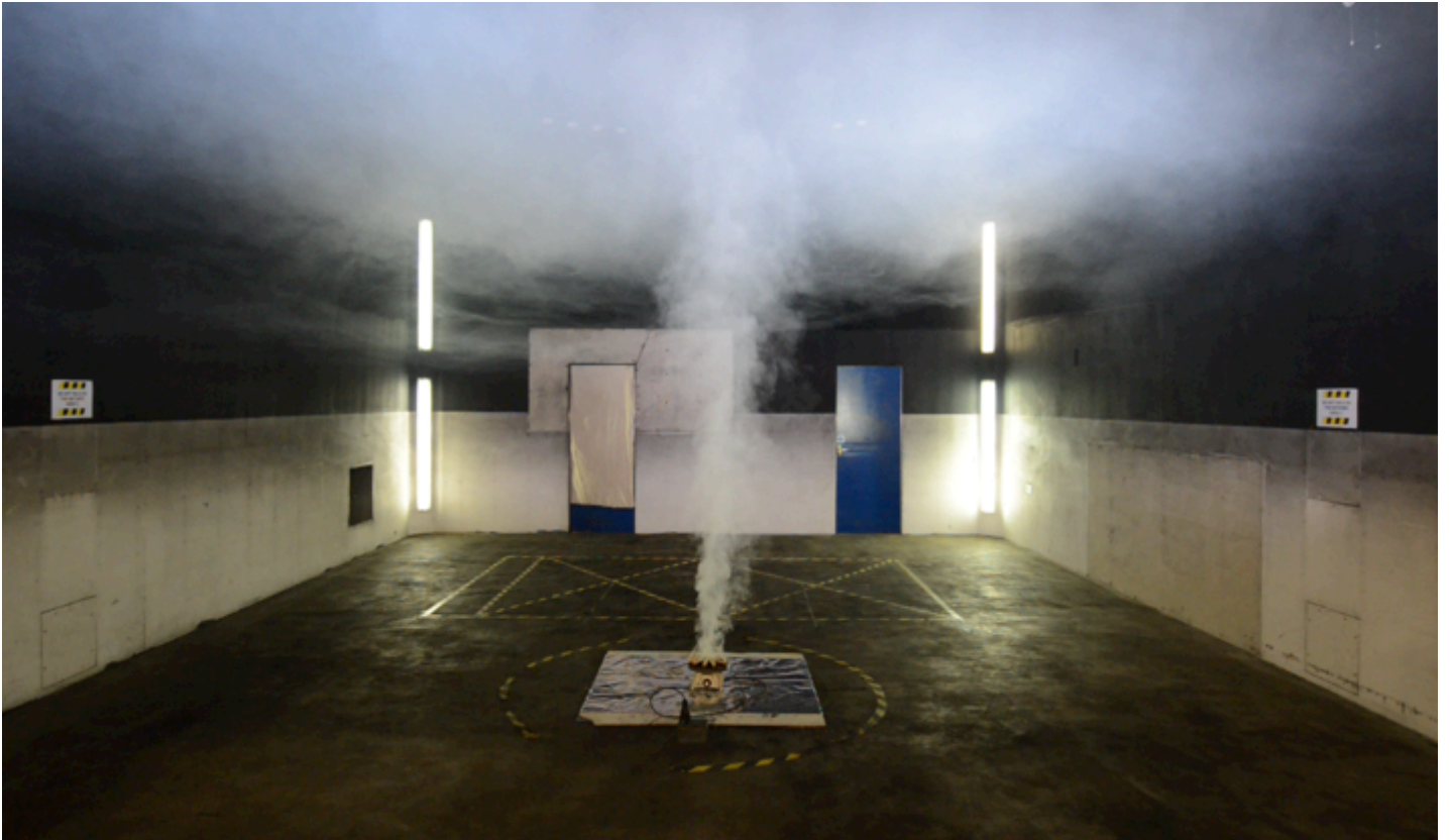
Figure 7: Tests 1 & 10- Smouldering beech wood sticks (TF2) in the fire test room
