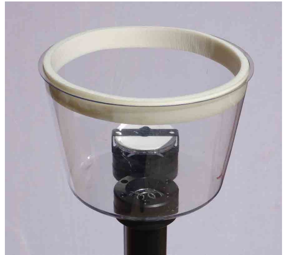
Figure 5: Trutest adapted using sticky foam to allow testing of domestic smoke alarms
