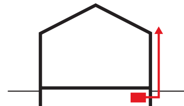
Externally constructed sump with high-level exhaust
