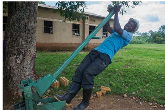
Cement-stabilised earth blocks are compacted in a manual press and cured in atmospheric conditions. (Image courtesy of HYT Uganda)
